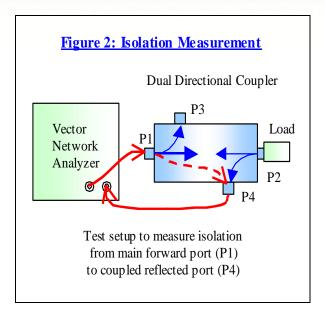
Per Figure 2, isolation is derived by stimulating the main forward port (P1) and measuring the output at the coupled reflected port (P4) with a good load on the main reflected port (P2). The coupler is then reversed to test the coupling factor. The main reflected port (P2) is stimulated while the output of the coupled reflected port (P4) is measured with the load connected to the main forward port (P1).
