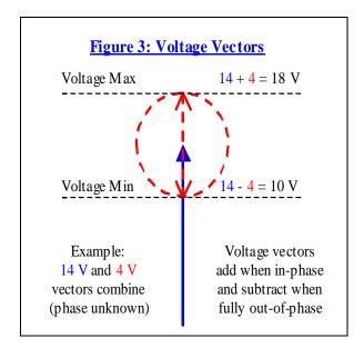
Once the minimum and maximum voltages are determined they can be converted back to power values. These forward and reflected power levels may then be used to calculate VSWR and Return Loss, including minimum and maximum values as well.
