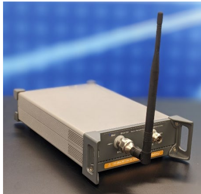
Figure 3: The Bird BNA100 hosting the antenna with a type N(m)-to-SMA(f) adapter in between.
