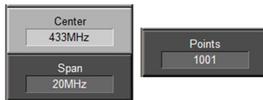
Figure 4: Use Stimulus->Center and Span options as well as Sweep Setup->Points to prepare for measurement calibration.
