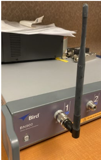
Figure 9: The DUT can be mated to the VNA with the adapter in between and measurement uncertainties can be accounted for by defining a port extension.
