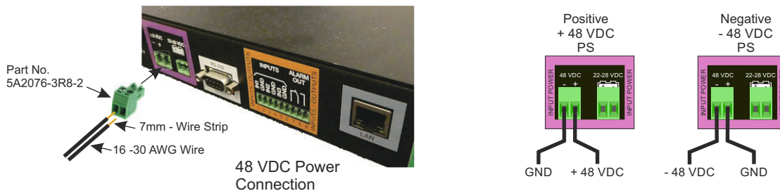
Figure 9 48 VDC Wiring Diagram
