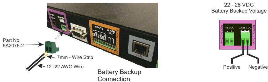
Figure 8 Battery Backup connector Installation
