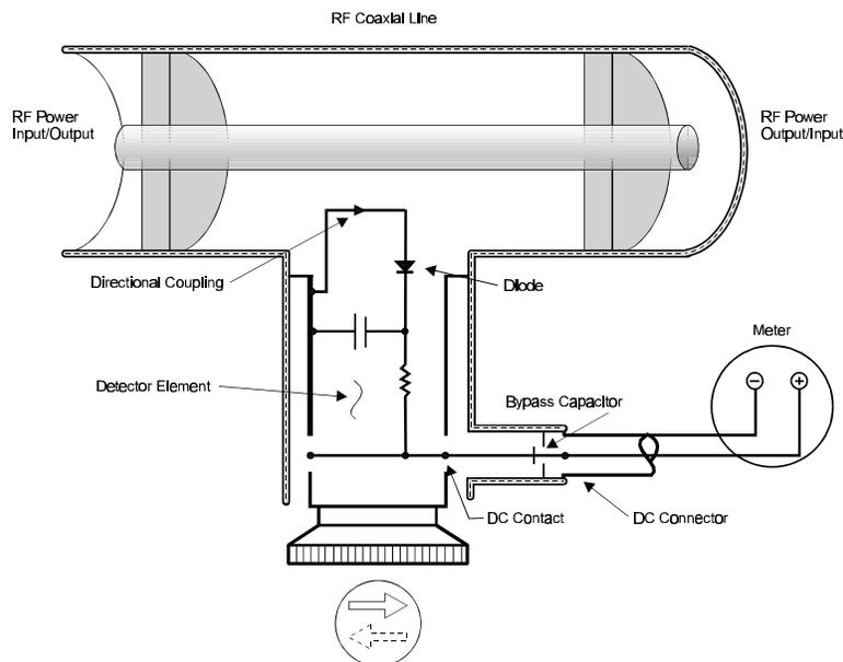
The forward wave travels and its power flows from the source to the load. It has an RF voltage  $E_f$  and current  $I_f$  in phase, with  $E_f / I_f = Z_0$ .
