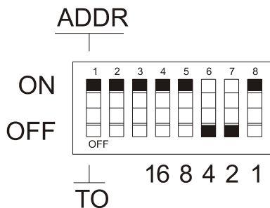
Figure 16 IEEE Interface Default DIP Switch Settings
