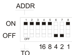
Figure 8 IEEE Interface Default DIP Switch Settings
