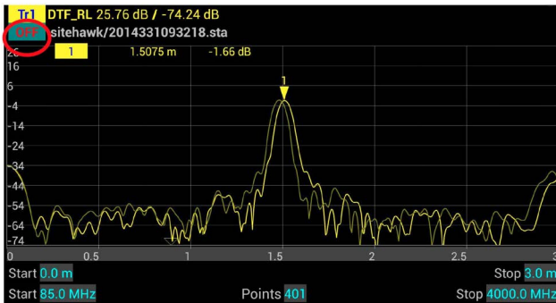
Figure 36 Recall Sta Data and Running Data
