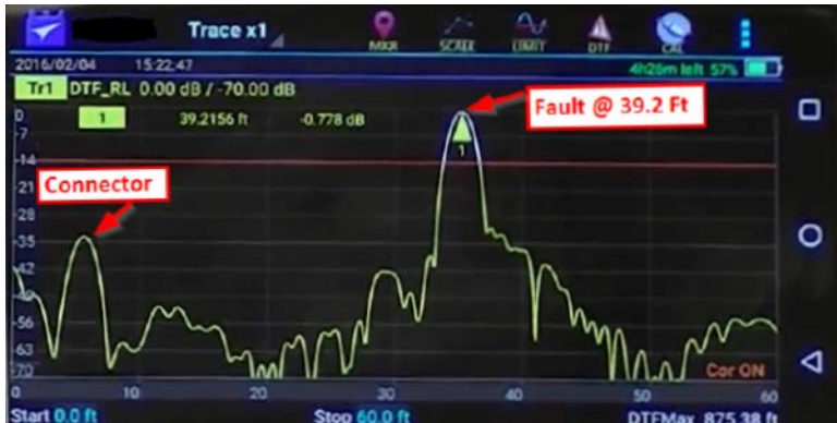
Figure 1 Typical Fault Location Measurement
