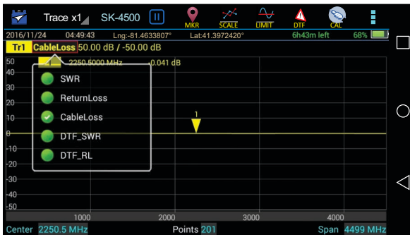
Figure 10 Selecting Cable Loss Measurement
